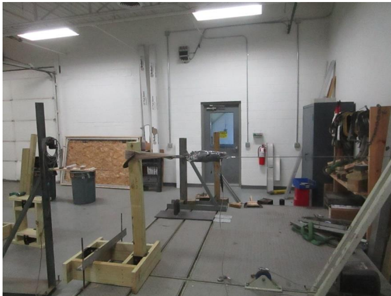
Photo No. 1 Load Applied Perpendicular to Rim Joist
