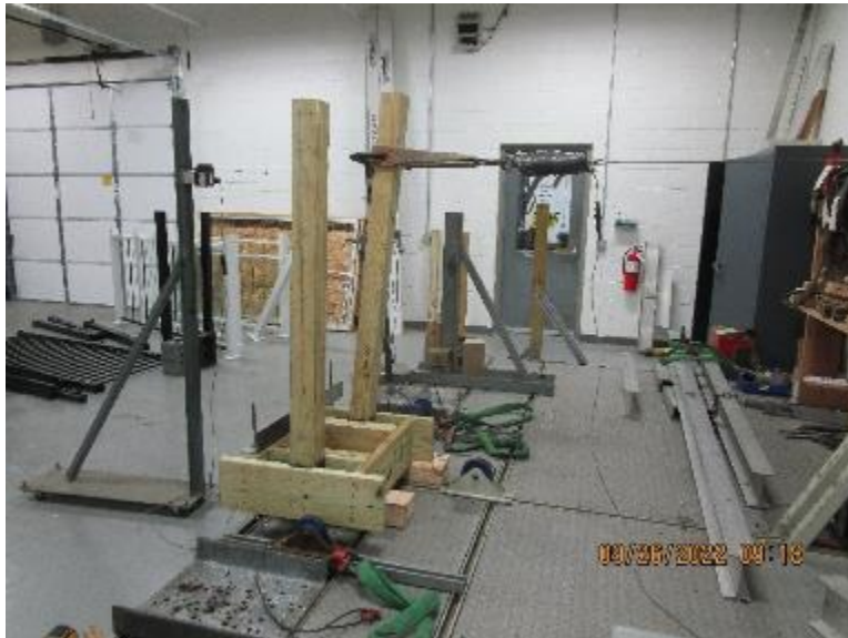
Photo No. 2 Load Applied Parallel to Rim Joist
